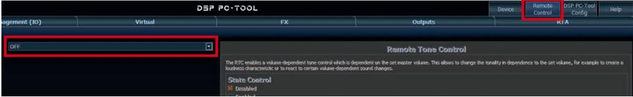
The subwoofer remote control is tied to the output channels that are supplied with one of the two virtual subwoofer signals (“Subwoofer 1” or “Subwoofer 2”) in the “Virtual to Output Routing” matrix. This can be any combination of output channels.
