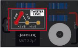
The crossover allows to optimize the level of the connected tweeter internally by repositioning the tweeter level jumper. Therefore open the crossover housing, pull the jumper straight upwards and reinsert it to the desired position.
