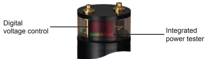
The integrated power tester is useful to determine voltage fluctuations easily. If the voltage supply is stable all LEDs are lighted up. In case of high voltage fluctuations the LEDs turn off from green to red.
