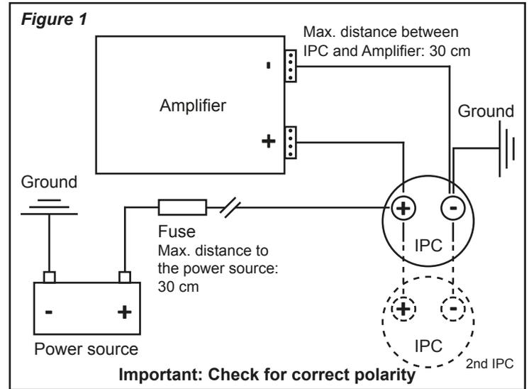
**Notice:** If your car audio system requires a higher capacitance you can install two or more capacitors in parallel. In this case you must connect the positive (+) terminals of all caps in a row and proceed the same way with all negative (-) terminals (see fig. 1).
