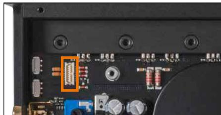
5. Insert the Allen screw which is delivered with the HDM into the mounting hole of the module and fix it carefully.
