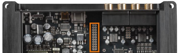
4. Make sure that the module is installed properly and all pins are fully inserted into the socket:
