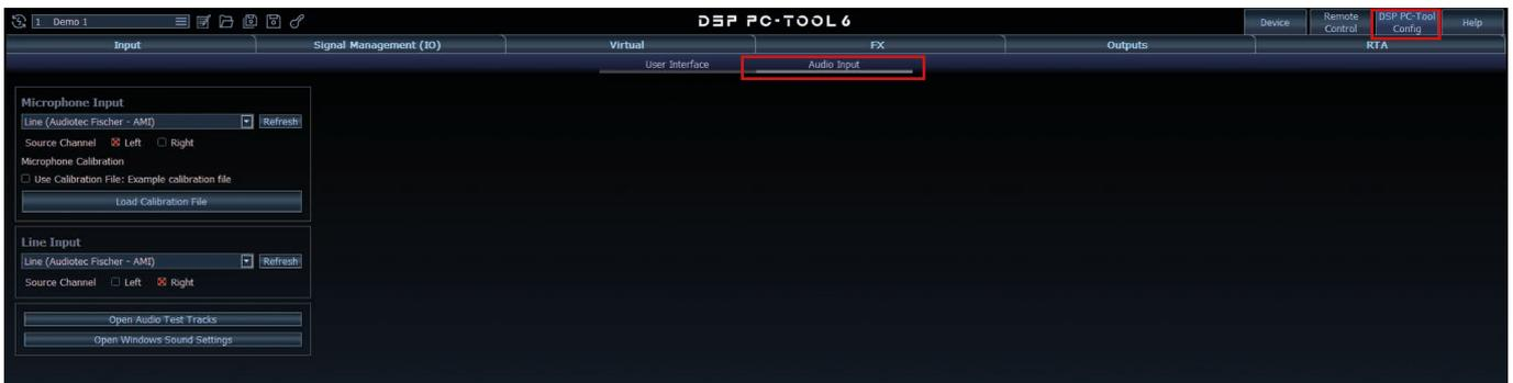
3. In the “Microphone Input” section, click “Load Calibration File”, then click “Extended Settings”, and select the appropriate calibration file from the included USB stick via the file explorer.
